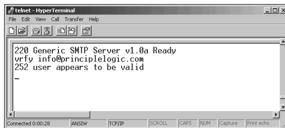
Figure 14-5: Using VRFY to verify that an e-mail address exists.
