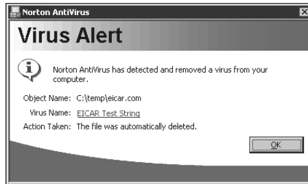
Figure 14-11: Using the EICAR test string to test antivirus software.
